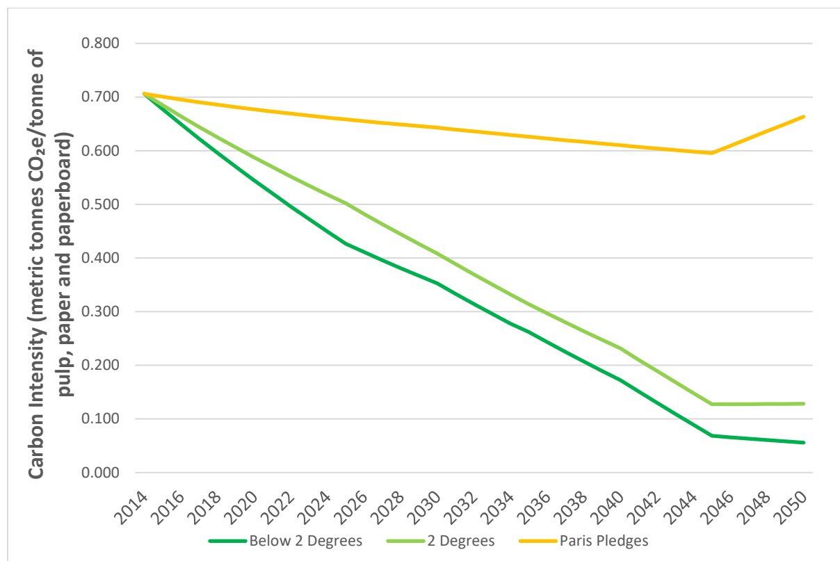
Figure 1. Benchmark global carbon intensity paths for the paper sector (tonnes of CO 2 e per tonne of pulp, paper and paperboard), consistent with limiting warming to below 2°C, to 2°C and with the sum of the Paris Pledges
